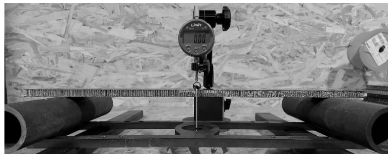
Fig. 3 Three-point bending experiment setup
