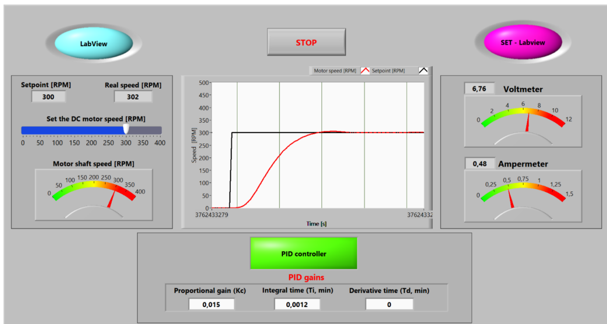
Fig. 2 GUI - graphical user interface in LabView
